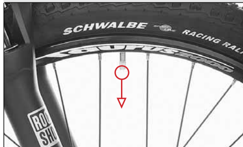
The valves must point directly towards the centre axis of the road wheel.
