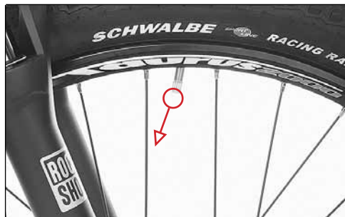
The valve does not point to the traversing wheel centre
