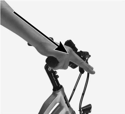
Figure 10. Brake lever aligned with the forearm.
