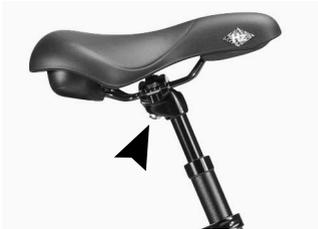
Figure 6. Saddle with one fitting block.
