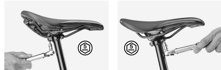
Figure 9. Steps for tightening/loosening the fitting blocks.
