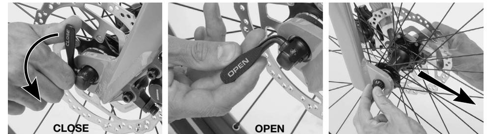
Figure 15. Opening the quick release axle.
