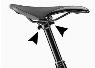
Figure 7. Saddle with two fitting blocks.
