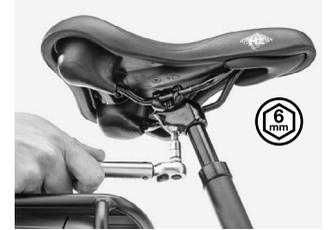
Figure 8. Tightening/loosening the fitting block.
