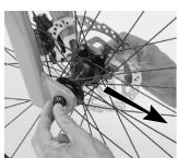
Figure 15. Opening the quick release axle.
