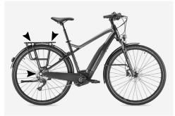
Figure 35. Fixing points for luggage racks with battery.
