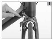
With an unapplied brake the brake pads should not be too close to the rim sides, otherwise they could drag along the rim during riding. Before making this adjustment, observe the notes in the chapter "Brake lever reach adjustment on SCOTT road bikes and SCOTT cyclo-cross bikes".
