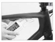
After cleaning and drying (a) check the chain for wear (b) and relubricate (c) (see the chapter "Bicycle chain" and the manuals of the component manufacturers).
