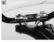
Make sure the saddle is clamped within the range of the marking on the saddle rail and not in the curved section of the saddle rails (c). Otherwise the saddle rail can fail! Check the bolts by using a torque wrench once a month according to the prescribed values.
