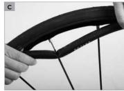
Make sure the inner tube does not get pinched and squashed between the tyre and the rim. You can prevent this by pushing the inner tube into the hollow of the tyre (c) with a finger as you work along.
