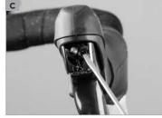
In the case of **SRAM** start by setting the cam disc on the slightly pulled and inward moved shifters. Screw in the screw positioned behind the hood in the body by using an Allen key **(e)**.
