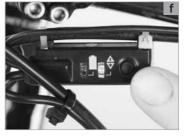
Continue turning the crank carefully and make sure the rear derailleur cage does not collide with the spokes and the chain does not move beyond the biggest sprocket. While doing so, press your thumb against the rear derailleur (a).
