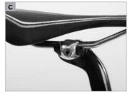
If you have a **single bolt system (c)**, the seat post for most of the sports saddles is designed for a saddle rail diameter of 7 mm.
