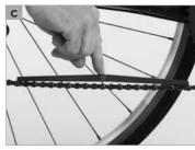
Replacing these components is relatively expensive compared with the costs of a new chain. It is therefore advisable to check the condition of the chain at regular intervals.
