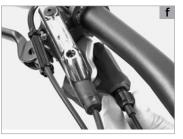
If the chain easily climbs onto the next larger sprocket, check whether it just as easily shifts to the small sprockets. If it does not, release the respective adjusting bolt a little. You may need several tries.
