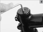
Check after the adjustment or assembly, whether the handlebars are firmly seated in the stem by trying to rotate the handlebars downwards (a). Verify whether the handlebar/stem-combination can be turned relative to the fork. Do this by taking the front wheel between your knees and trying to twist the handlebars. If there is movement, carefully tighten the bolts a little more and check again the proper fit (b).
