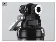
When you have set the sag correctly, as above described, and when the rear shock works properly during a normal test ride, but if then the rear shock bottoms out nevertheless, you can increase the compression damping a little.
