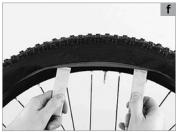
After levering a part of the tyre bead over the edge of the rim you should normally be able to slip off the whole tyre on one side by moving the tyre lever around the whole circumference.
