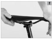
If you have a single bolt system (a), the seat post for most of the sports saddles is designed for a saddle rail diameter of 7 mm. Replacement outer clamps for ovalized saddle rails of 8 mm  $\times$  8.5 mm (W  $\times$  H) as well as for carbon saddle rails bigger than 8 x 8.5 mm are also available. If you are not sure which saddle rail type you have or if you need further information, contact your SCOTT dealer.
