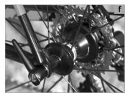
Hold the lock nut on the right side of the hub tight. Turn the RWS quick-release lever clockwise to pre-tighten the RWS system. Depending on the fork mounted or the frame model, the number of turns you need varies. You need at least six, in most cases however more turns. During the first turns you should be able to turn the RWS quick-release lever nearly without resistance.
