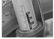
To measure the travel you can use the rubber ring mainly located on the thinner, plunging tube of the suspension fork. If there is no rubber ring, tie up a cable tie around one of the stanchion tubes. Make sure it is not too tight, you should still be able to move it, it should however not slip by itself.
