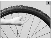
To make sure the inner tube does not get pinched between the rim and the bead, move the tyre sideways back and forth between the sides of the rim. While doing so, also check whether the rim tape has shifted.
