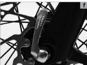
When continuing to close the lever the resistance you feel should increase significantly and towards the end even more strength is required to close the lever. Use the ball of your thumb while your fingers pull on an immovable part, such as the fork (a) or a rear stay, but not on a brake disc or spoke, to push it in all the wav.
