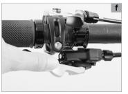
Pulling the small lever located in front of the handlebars from the rider's view-point and actuated with the index finger (index finger lever) (a) shifts the chain towards the smaller chainwheels/sprockets, i.e. on the right side to the higher gears and on the left side to the lower gears.
