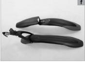
Retrofittable mudguards for fix fastening are usually made of plastics and are secured in the correct position by means of additional stays. The length of the stay is perfect when the bottom edge of the mudguard runs at an approx. distance of 15 mm parallel to the tyre. Also make sure neither the brakes nor the steering are affected.
