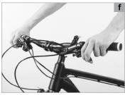
With disc brakes you should have a stable pressure point at once. If you have to actuate the brake lever more than once to get a positive braking response. have the SCOTT bike checked by your SCOTT dealer immediately.
