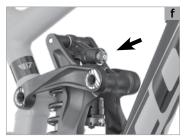
Always make a test ride over different terrains with various surfaces after each change to the setting. Check afterwards the position of the rubber ring/cable tie. Its distance from the wiper is the maximum rear shock travel that you have used.
